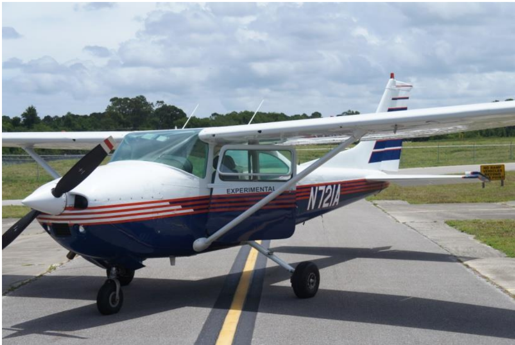
Figure 1: Cessna 182 adapted into a Surrogate UAS to support research and testing.
