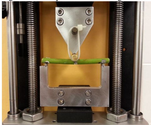
Figure 3. Small scale three point bend test equipment
