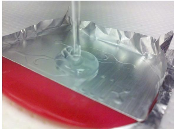
**Figure 5:** Cutaway view of foil master with PDMS. The PDMS is typically poured closer to the master surface to avoid entraining air bubbles. The turned edges of the foil on all sides form a vessel to contain the liquid PDMS during the curing stage.
