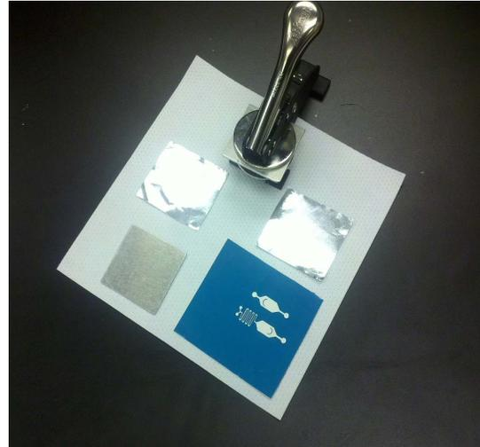
**Figure 2:** Clockwise from top. The hand-embosser with custom top pressure plate affixed. Top foil layer (backing). Cerulean vinyl (ABM) with Silhouette-cut pattern peeled, revealing white backing. Bottom pressure plate not affixed. Bottom foil layer (embossed layer).
