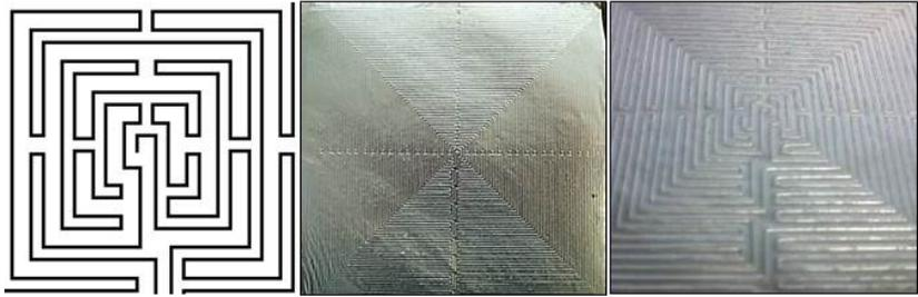
**Figure 7:** Large area emboss pattern. Center section of an AutoCAD drawing of seven nested Chartres-like labyrinths occupying a 5.75 inch<sup>2</sup> area (Left). The embossed labyrinth pattern using a modification of the methods described on a heated Carver® press, also 5.75 inch<sup>2</sup> (Middle). A zoomed view of the middle of the nested labyrinth more clearly showing the channels, which are approximately 500 microns wide.
