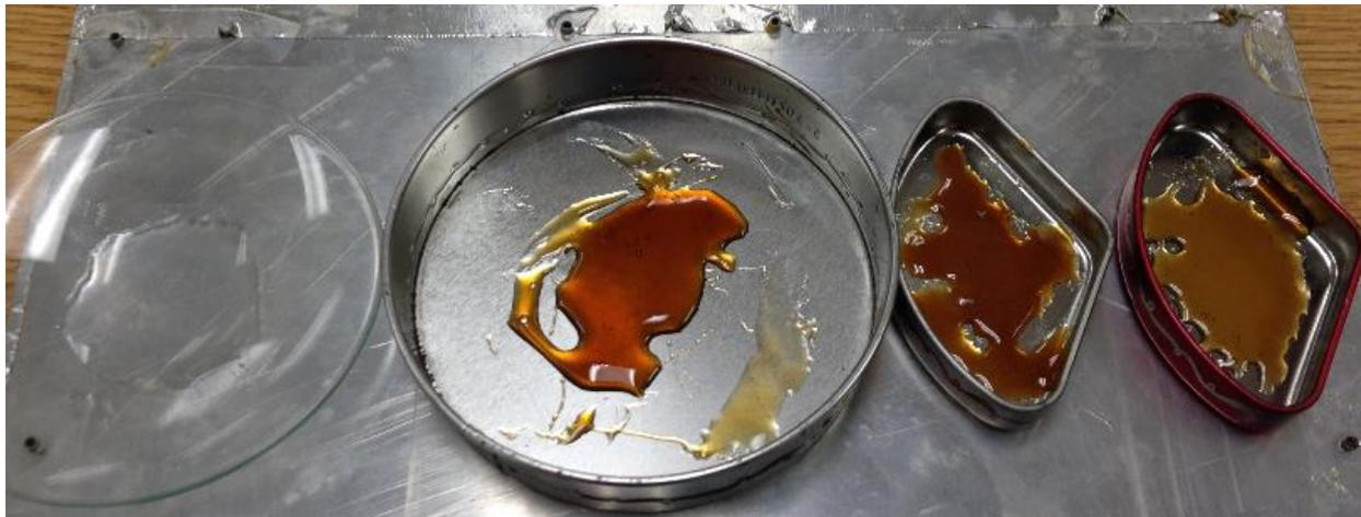
Figure 2. PLA samples polymerized from: synthetic lactic acid, malt, wort, and spent grain (from left to right).
