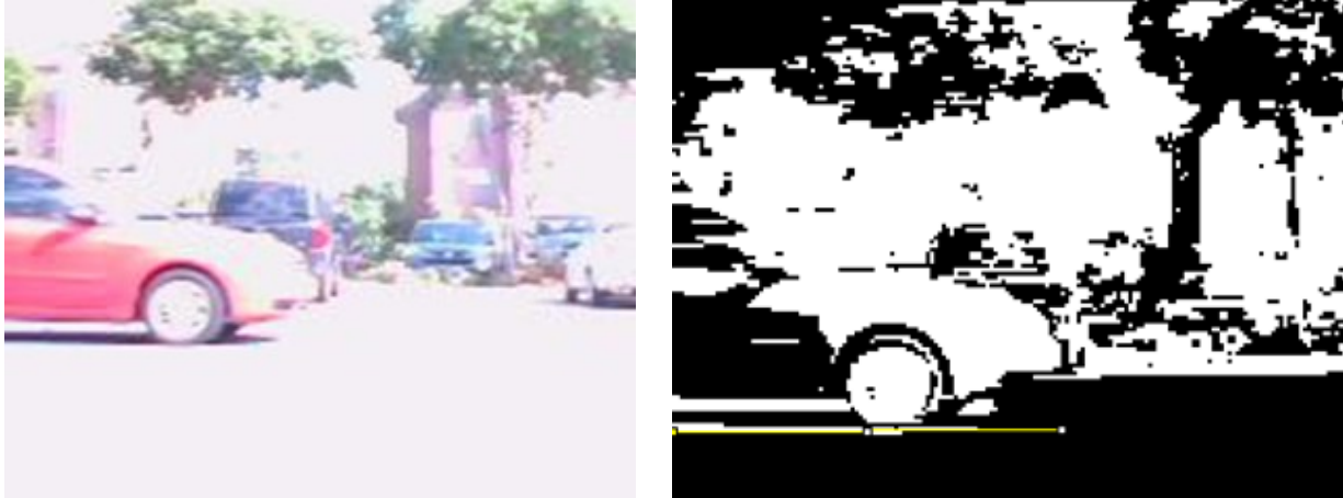
Figures 1 and 2. Original image and image after thresholding is applied
