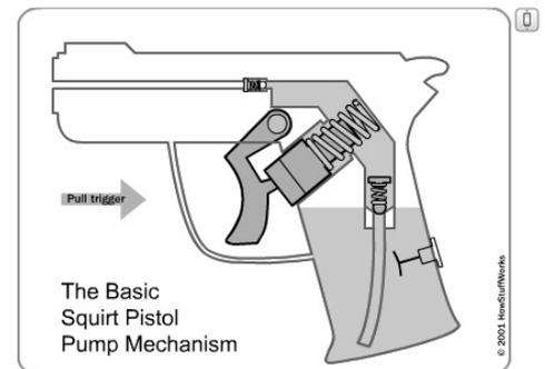
Figure 1—The Basic Squirt Pistol Pump Mechanism [2]
