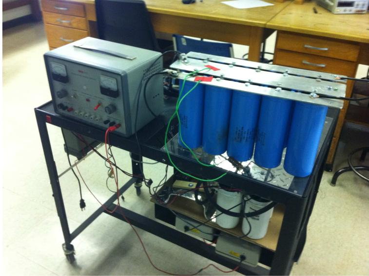
Figure 4: Prototype of EM can crusher
