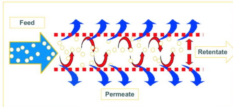
Figure 3. Schematic showing the principles of crossflow filtration [32].
