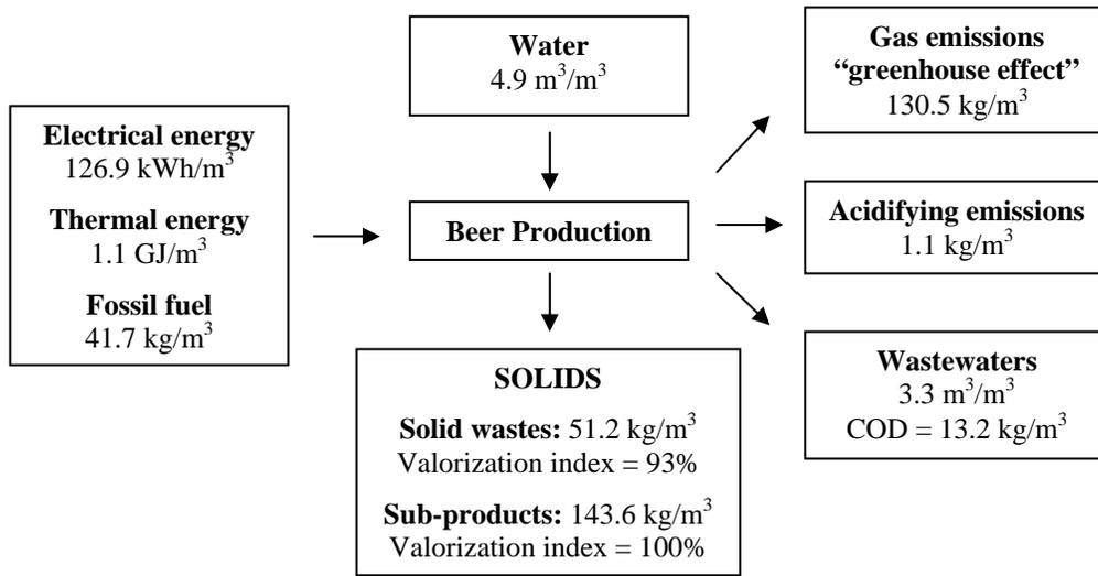
Figure 2. Mass balance applied to Unicer SA breweries representing specific values, i.e., values per m<sup>3</sup> of produced beer [13].
