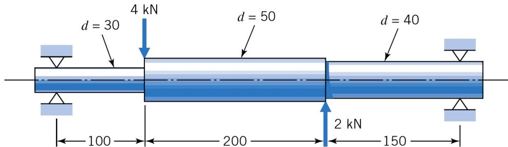
Figure 1: Stepped Shaft (all dimensions in mm) [17]
