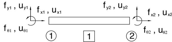
Figure 3: Schematic of beam element [18]
