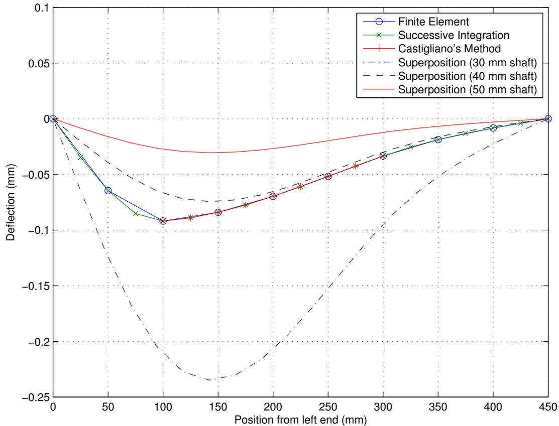
Figure 5: Comparison of methods for calculating shaft deflection
