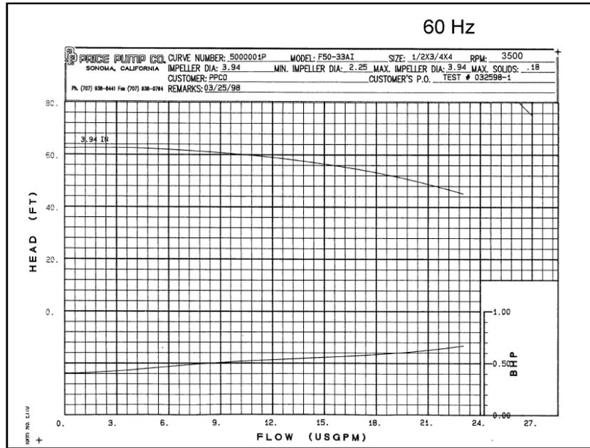
**Figure 2: Manufacturer's Pump Curve [1]**
