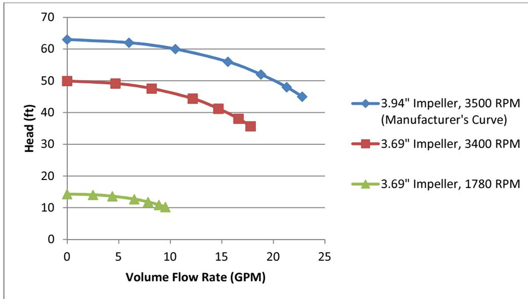
**Figure 3: Manufacturer's Curve and Predicted Curves**
