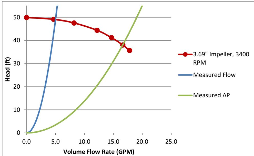
**Figure 4: Pump Curve and Operating Point**
