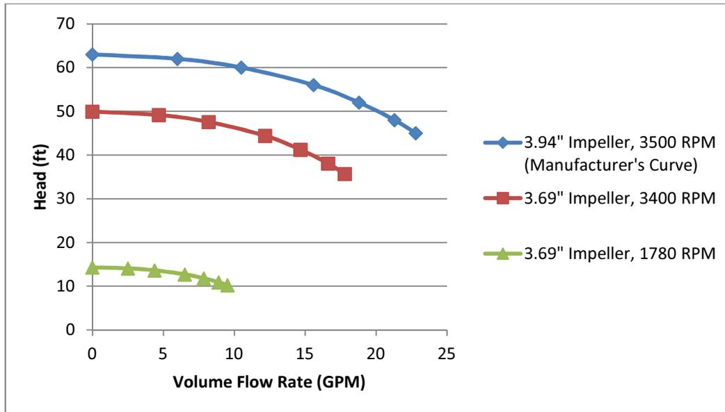
**Figure 3: Manufacturer's Curve and Predicted Curves**
