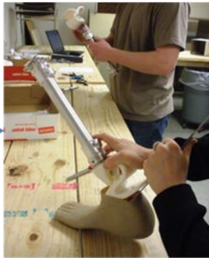
Figure 4. Fitting skin into foot.
