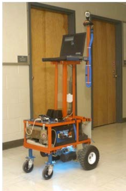
Figure 2. An early prototype of SPARC's Tourbot – a tourguide assistant robot.
