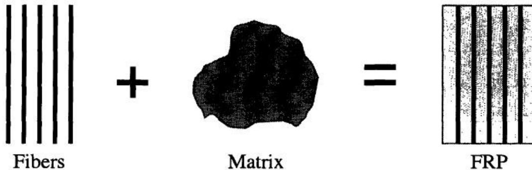
Figure 2: Fiber-Reinforced Polymer Breakdown
