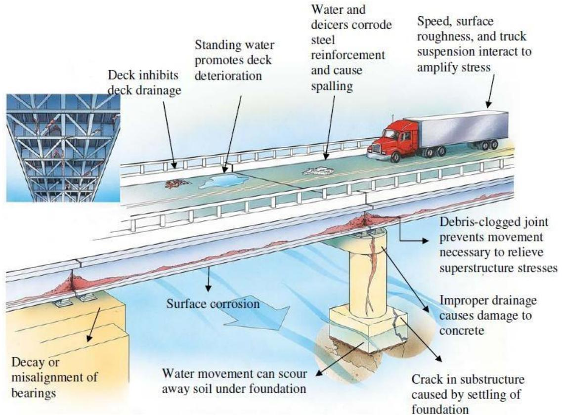
Figure 1: Corrosion Causes
