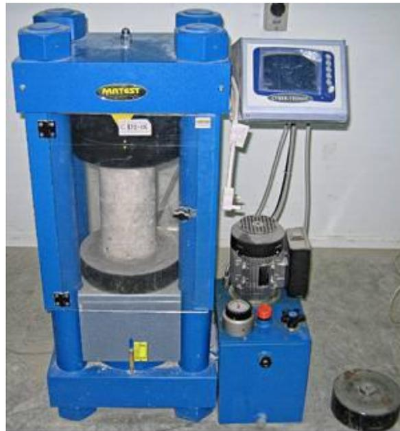
Figure 5: Compressive strength test of concrete.
