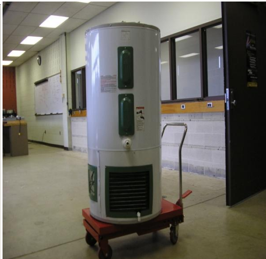
Figure 2: Field Test Unit: Dehumidifying Water Heater
