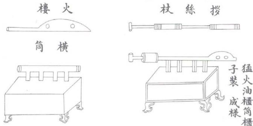
Figure 6 Components of the Chinese Flamethrower (Fierce Fire Oil Projector)
