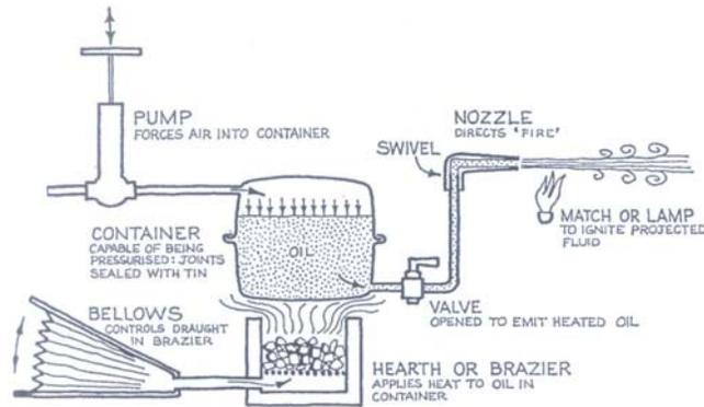
**Figure 1: Shipboard Byzantine Flamethrower**
