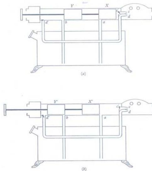
**Figure 4** Needham’s proposed solution to the Chinese flame thrower
