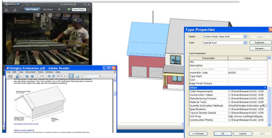
**Figure 4: Retrieved manufacturing video and estimation guidelines for Asphalt Shingles roof component**
