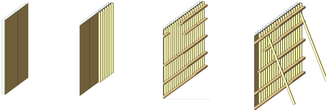
**Figure 5: Erection sequence of wall formwork system**
