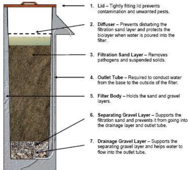
**Figure 3. Parts of a BSF**
