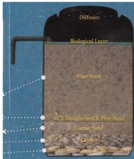
**Figure 4. Modified BSF Schematic**
