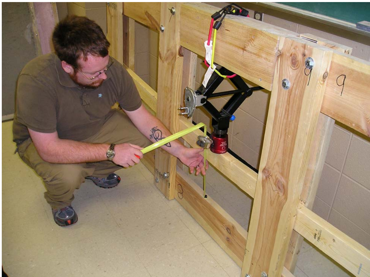
Photograph Three: Beam Bending, Laboratory Setup
