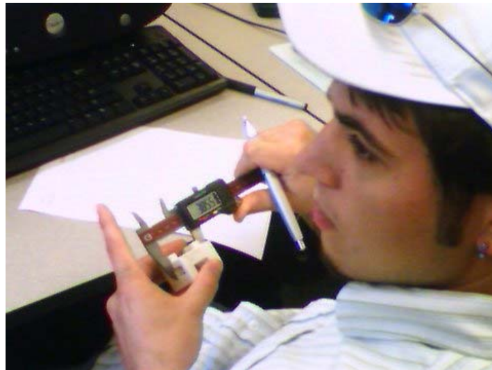
Figure 2. Student measuring a part with digital calipers during Module 1 in the ENGR 1170 lab.
