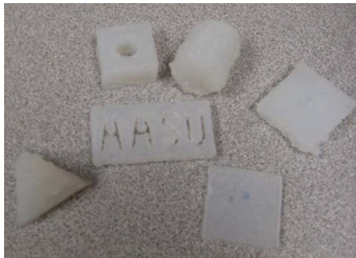
Figure 6. Examples of fabricated parts using the Fab@Home kit
