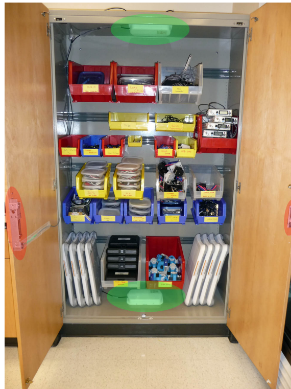
Figure 2. RFID smart cabinet housed in the laboratory. Antennas are housed on the top and bottom of the cabinet as highlighted in green. The electric lock (left) is driven by the reader input / output ports and includes a magnetic reed switch (right) to activate only when the door is closed, both highlighted in red.
