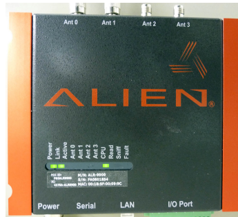
Figure 1. RFID reader used for tag identification. This reader communicates via local area network (LAN) and includes input output ports that allow for control of automated access control.
