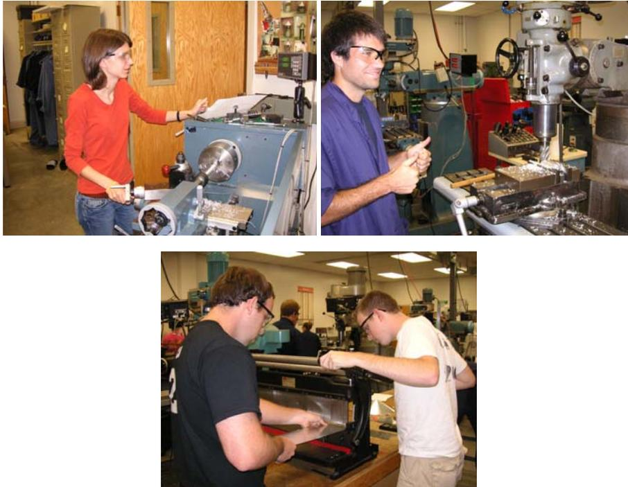
**Figure 1. Students work at a lathe, milling machine, and press brake**
