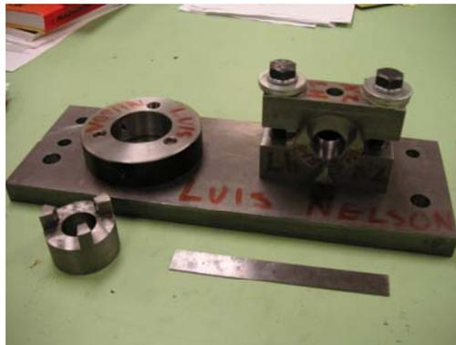
**Figure 7. A completed fixture with the fabricated part**
