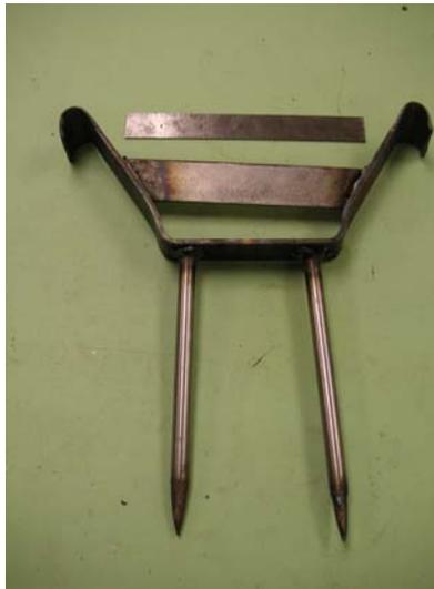
**Figure 3. Welding shop practical exam: boot scraper**
