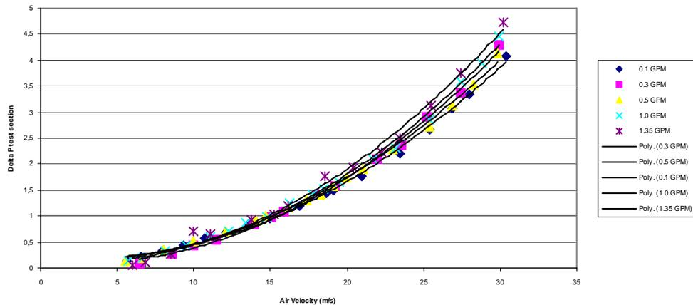
Figure 13: Ground test. Test section pressure drop for concurrent gas-liquid flow in the 3/4 inch horizontal pipe (pressure drop in the test section is measured in Psi).
