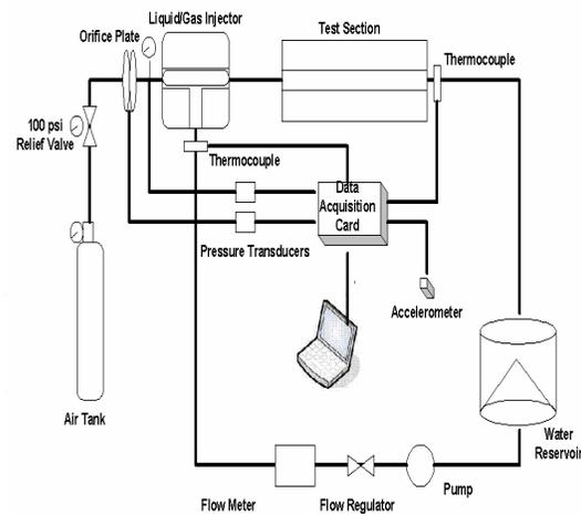
Figure 12: Diagram of experimental apparatus
