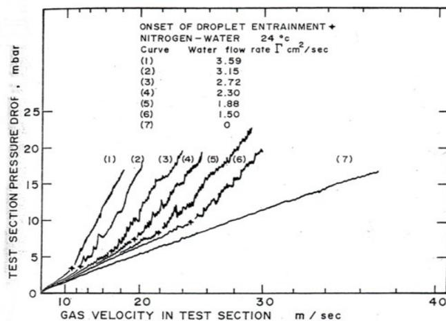
Figure 11 : Test section pressure drop for concurrent gas-liquid flow with onset of droplet entrainment [4]
