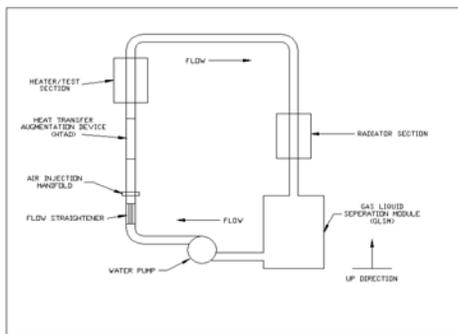
Fig. 1. Schematic of the Water Flow Loop
