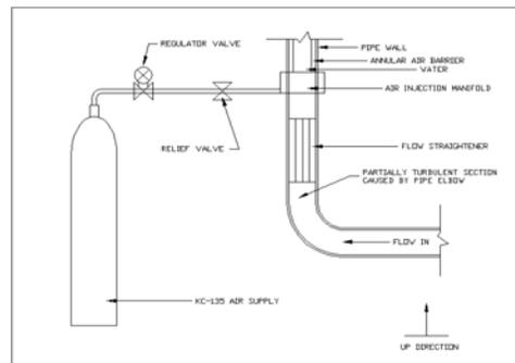
Fig. 2. Schematic of the Air Injection System
