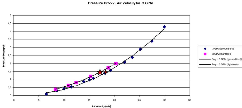
Fig. 15: Critical velocities (★microgravity, ✦ microgravity) at the onset of entrainment (water flow rate: 0.3GPM )
