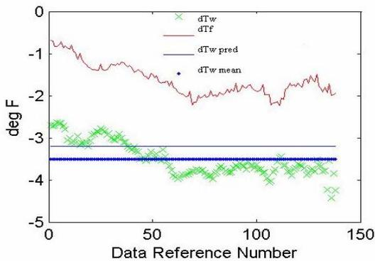
Fig. 9. History of the temperature difference of the fog and water for reduced gravity condition
