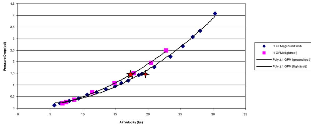
Fig. 14: Critical velocities (★ microgravity, ✦ microgravity) at the onset of entrainment (water flow rate: 0.1GPM )
