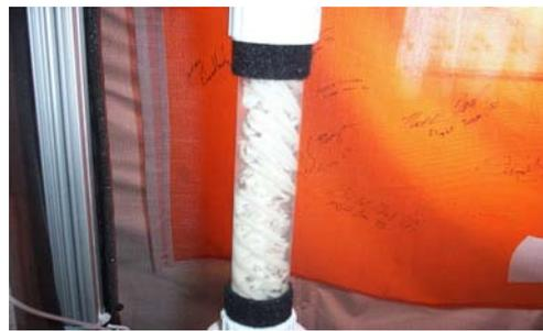
Fig. 4. Flow with swirling-helical HTAD
