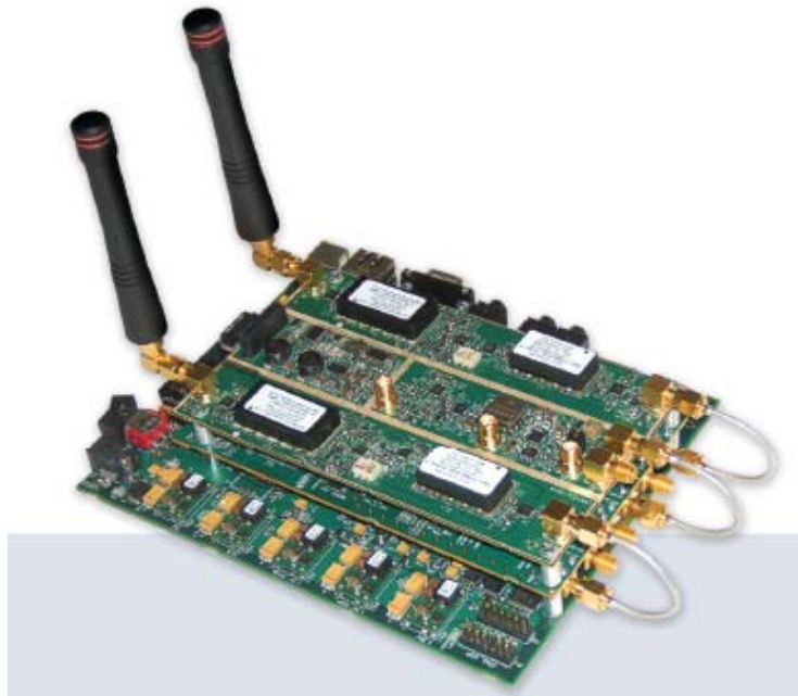
Figure 1 - SFF SDR from Lyrtech [1] which features an Xilinx SX35 [2] user programmable FPGA.
