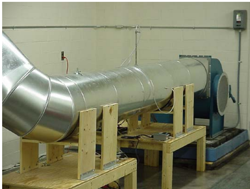
Figure 1. Laboratory set-up for one of the course's four problems. The undergraduates must take pressure and power measurements for several different settings of inlet guide vanes on a centrifugal fan.
