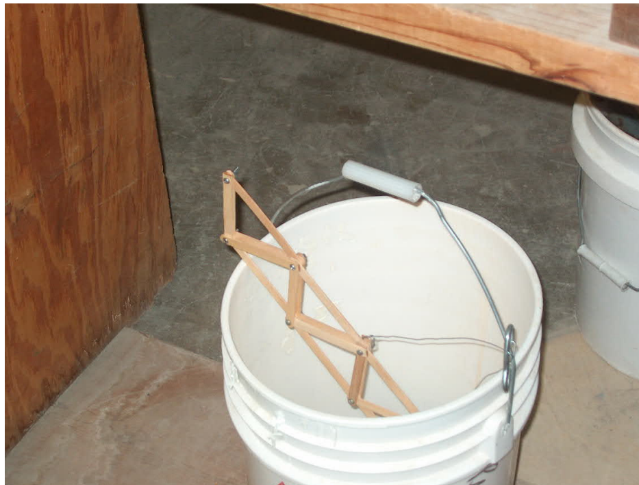
Figure 4. Broken truss bridge in bucket following load testing
