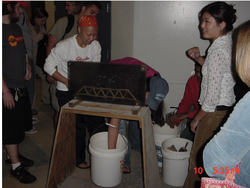
Figure 3. Frame holding a truss bridge about to be load tested
