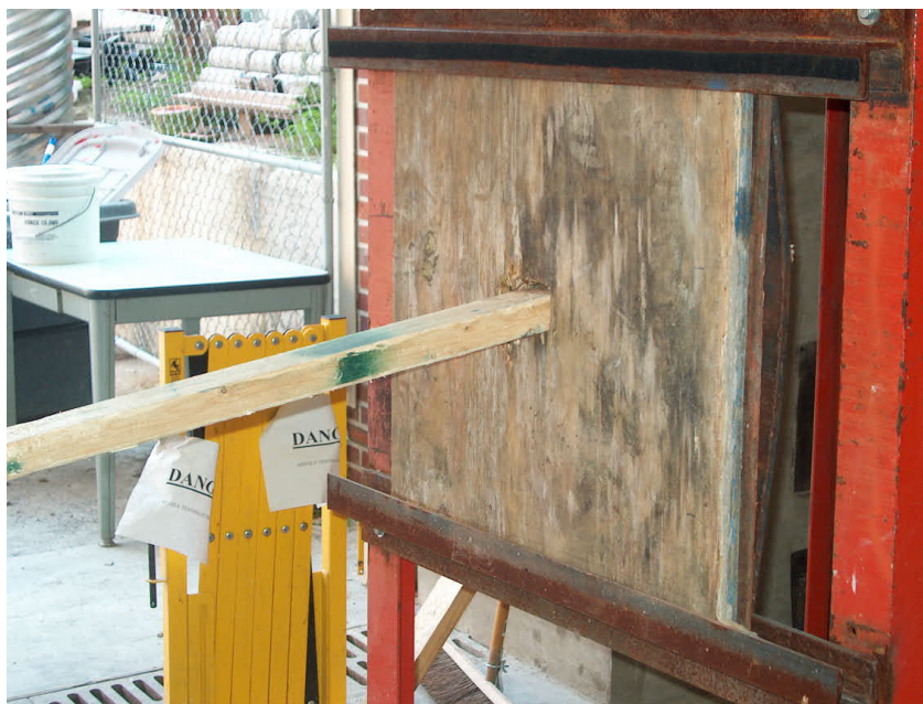
Figure 6. A 2-in. by 4-in., 9-ft long piece of wood shot by the air-pressure cannon (to simulate category 1 hurricane or 75-mph force winds) penetrated into a 2-ft by 2-ft by \frac{3}{4} -in. plywood attached to a steel frame
