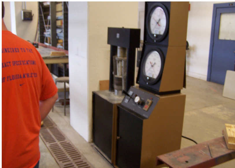
Figure 7. Determination of compressive strength of concrete cylinder
