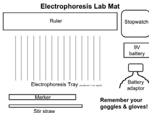
Typically, it takes less than an hour before the class to set up stations for 40 to 50 students. Placing all of the equipment on "lab mats" helps facilitate this process. A sample Electrophoresis Lab Mat is shown.
