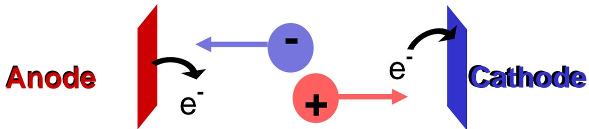
We are going to measure the **mobility, or rate of migration**, of NaCl ions in a water filled tray. Mobility,  $\mu$ , of a charged ion is described by
