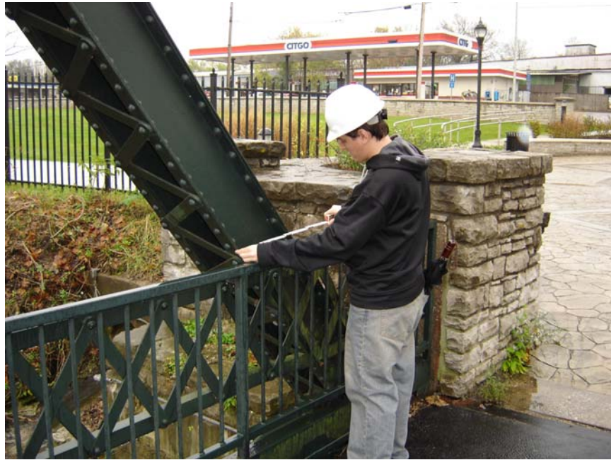
Figure 4: Engineering Student Measuring Section Properties of a Truss Diagonal
