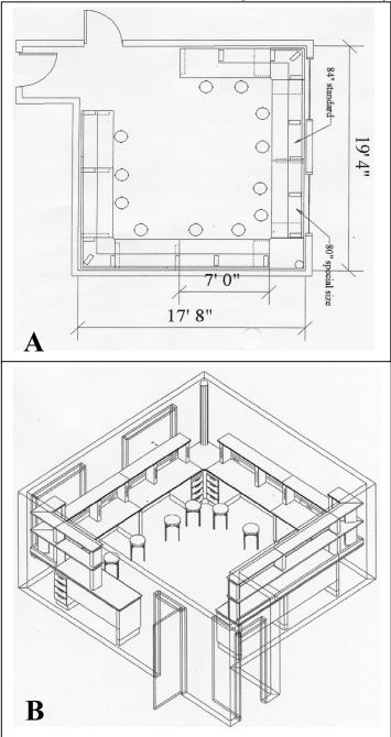
Renovation plan for the shared laboratory. Panel A shows the adopted floor plan while Panel B shows the room elevation plan with cabinets, desks and shelving. The room is designed for seven student pairs (14 students).
