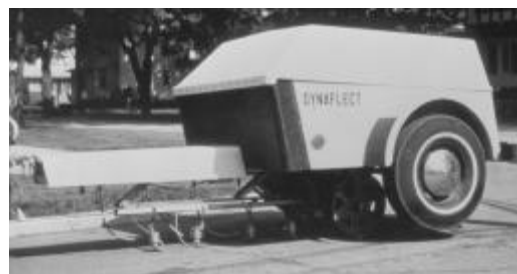
b) Dynaflect machine performs a non-destructive sub-surface condition survey
