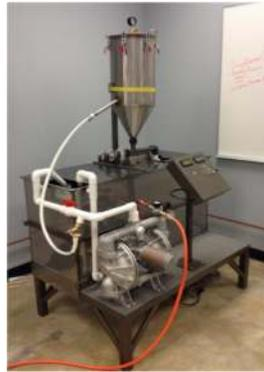
**Figure 2: Erosion Test Fixture**
