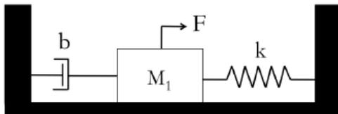
Figure 1- Spring-Mass Damper System
