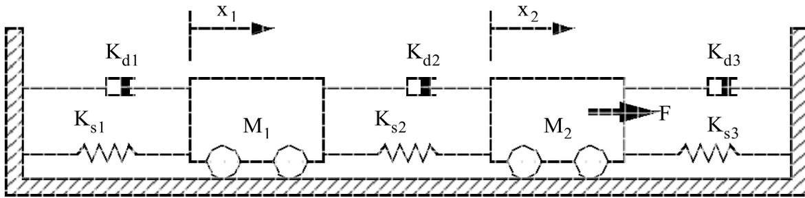
Figure 4- Two degree of freedom mechanical system-Example 2<sup>[4]</sup>
