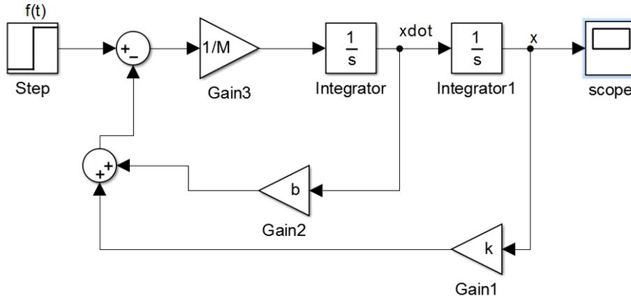
Figure 2- Simulink Model for System in Example 1
