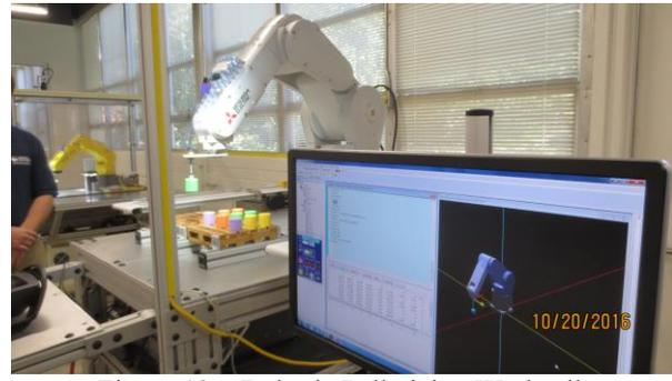
Figure 13 – Robotic Palletizing Workcell
