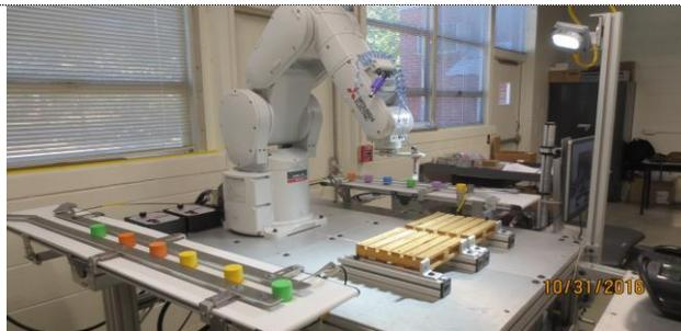
Figure 9 – Mitsubishi RV-7F Robot and conveyor layout
