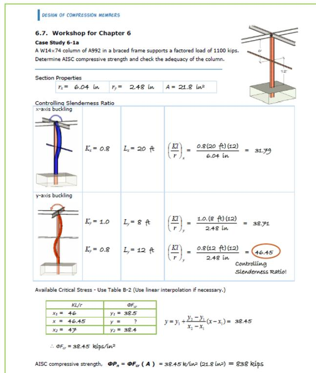
Figure 2 Column Buckling Visualized in 3-D Space
